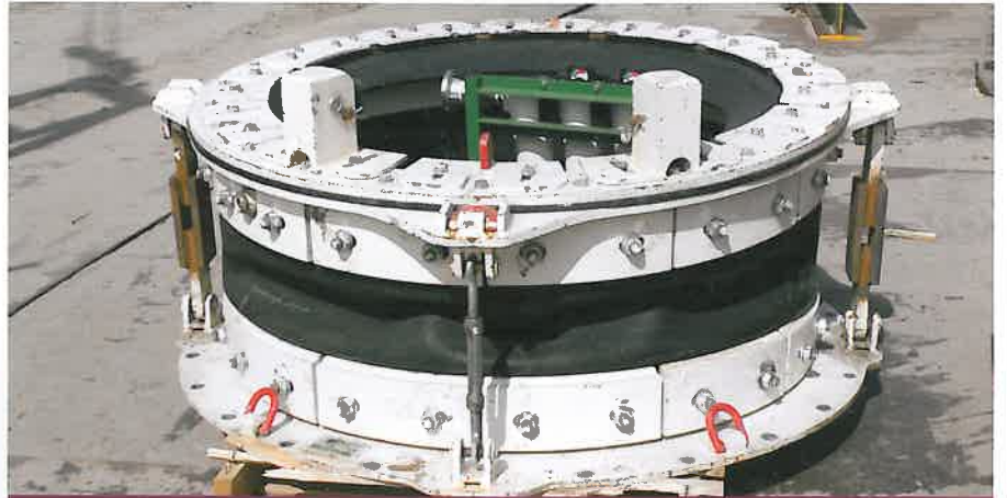
The seal, through which the pipe is thrust, that is used in the launch pit to prevent the Bentonite slurry leaking out.
