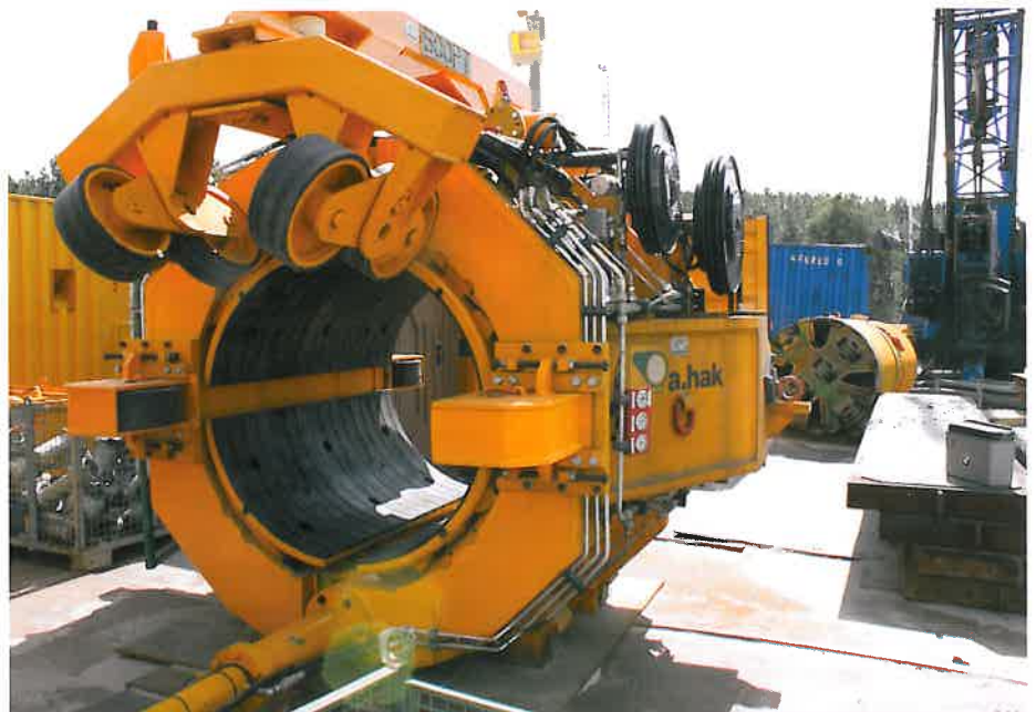
The Herrenknecht 500 tonne clamping unit that will be used to push the pipe into the microtunnel.
